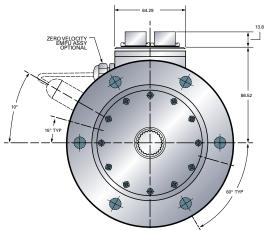
**Outline Dimensions (SI Units)** MCRT® **Maximum Overhung Moment** Model **Torque Range Spline Data** Dimension L All 16 teeth, 20/30 D.P., 30° Pressure Angle 48850V 452 N-m 218 ΑII 48851V 452 N-m 24 teeth, 20/30 D.P., 30° Pressure Angle 231
