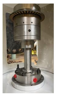
changes manifest in more than just differences in pressure and flow; they impact power, efficiency, and ultimately the axial thrust developed during operation. Having real-time axial thrust data can be an important piece of a successful condition monitoring strategy. By monitoring critical pump and motor data, end users are empowered to be more predictive in their approach to maintenance by detecting emerging problems and making the best possible decision for their equipment and plant.
