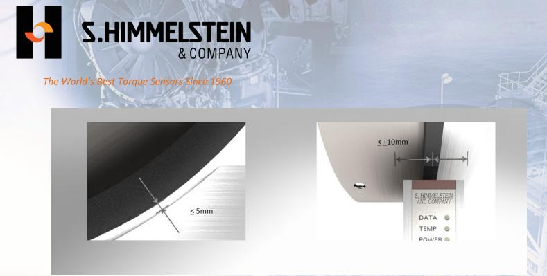
When installing the sensor, first install the rotor/flange into the system driveline, then slowly approach the powered stator housing from any direction and angle to the antenna at the edge of the flange until the indicator lights on the stator show green. The sensor is then ready to enter the normal operating condition.
