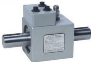
Torque and Speed requirements are readily met with Himmelstein's low cost [MCRT® 48200V](#) Compact Digital Torquemeters equipped with a zero velocity speed pickup. They output torque in digital and analog form and speed as a pulse train. In summary:
