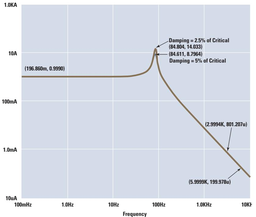
Figure 6. Frequency Response of Competitive 3kNm Torquemeter With Low Damping.
