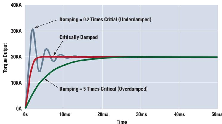
Figure 4. Response to Step Input With MCRT 87007V(25-3) Torquemeter Installed.
