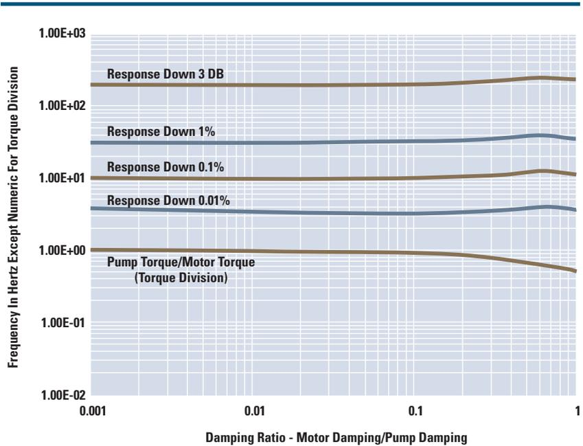
Figure 5. Effect of Damping Ratio on Frequency Response and Torque Division.
