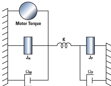
Figure 1. Driveline Mechanical Schematic
