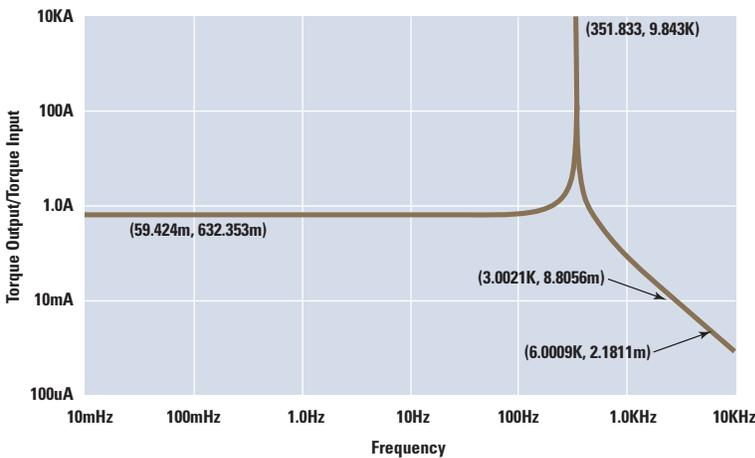
Figure 3. Computer Solution With Damping Set to Zero -  $R_m = R_p = 10^{+15}$  ohms  $\approx$  Infinity.
