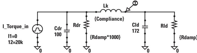
Figure 2. Electric Analog of Driveline
