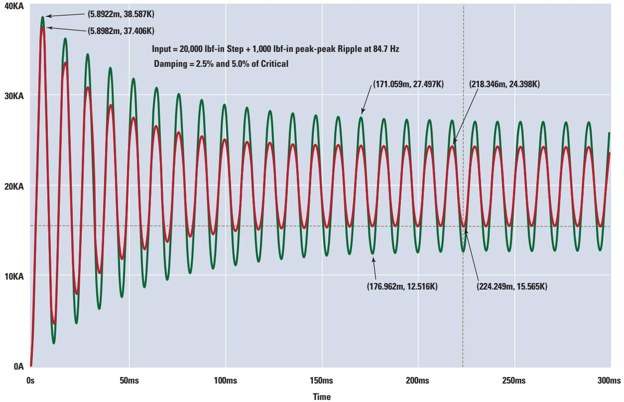
Figure 7. Competitive 3 kNm Device Response to Step + Ripple at Drive Natural Frequency
