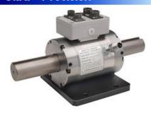
MCRT® 48800V & 49800V Ultra Precise Shaft Torquemeters have analog and digital inputs and the highest accuracy of any similar torquemeter. Features include: Capacities from 25 to 375,000 lbf-in, Output Torque, Speed & Power in Analog & Digital Form, 400% Overload and 300% Overrange, and 0.02% Combined Nonlinearity and Hyst-eresis. Contact us for more information.
